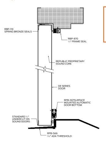
Republic STC systems can include: threshold, adjustable head and jamb seals (soffit mounted), stationary seals at door rabbet, surface mounted auto door bottom and Cam-lift hinges. Reference republicdoors.com for details and cut sheets.
